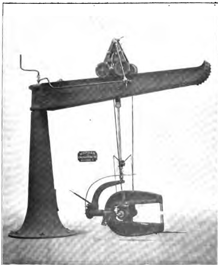
Fig. 54.—PORTABLE HYDRAULIC RIVETER.
